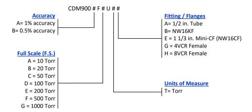
Example: CDM900BFAUTB (CDM900, 0.5% accuracy, 10 Torr F.S, Torr units of measure, NW16KF fitting)
